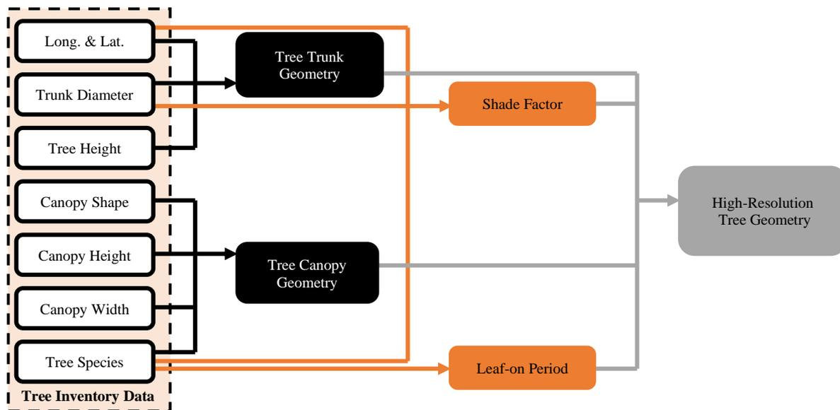
Figure 1: Overview of the framework for creating high-resolution tree geometries for use in urban energy modelling simulations
