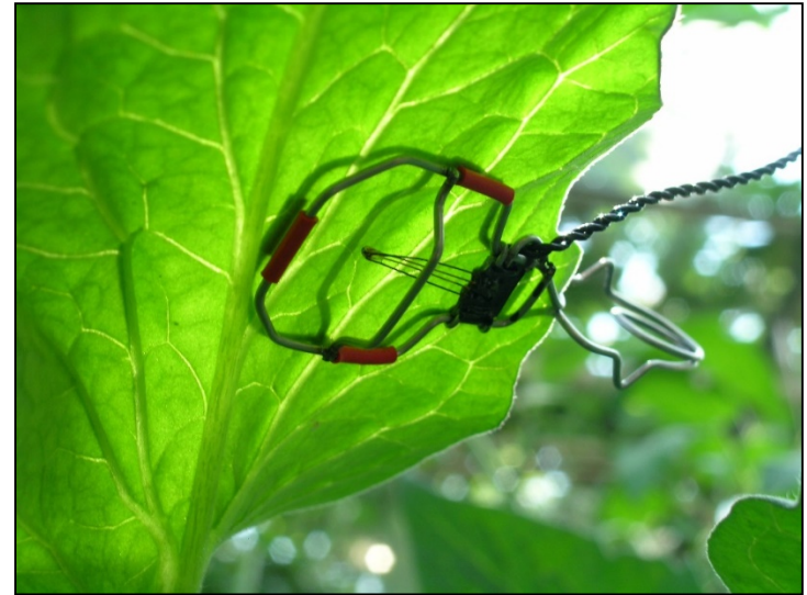
Leaf temperature probe used to measure absolute temperature of a leaf. Note: This study relied on previously published leaf temperatures. (Image from www.envoglobal.com .)
